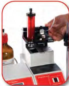
Interchangeable burette assembly with intelligent volume recognition system. Simply remove the retaining screw, slide out the burette assembly and replace with different volume or titrant burette.
